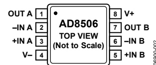
Figure 1. 8-Lead MSOP (RM-8)
